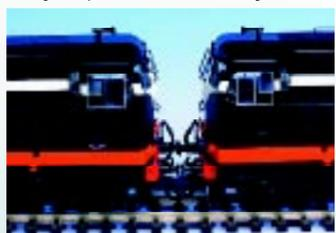
When running in multiple, Roco close couplers can be used to bring the locomotives really close together.
